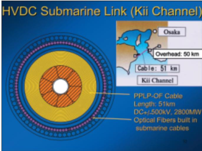
This cable handles the highest power for submarine use thus far. Several fibers housed in steel pipes are incorporated in the outer layer of the cable for information transmission as well as sensing damage to the cable. Total length of the DC link is slightly over 100km, of which the portion of submarine cable is about half.
