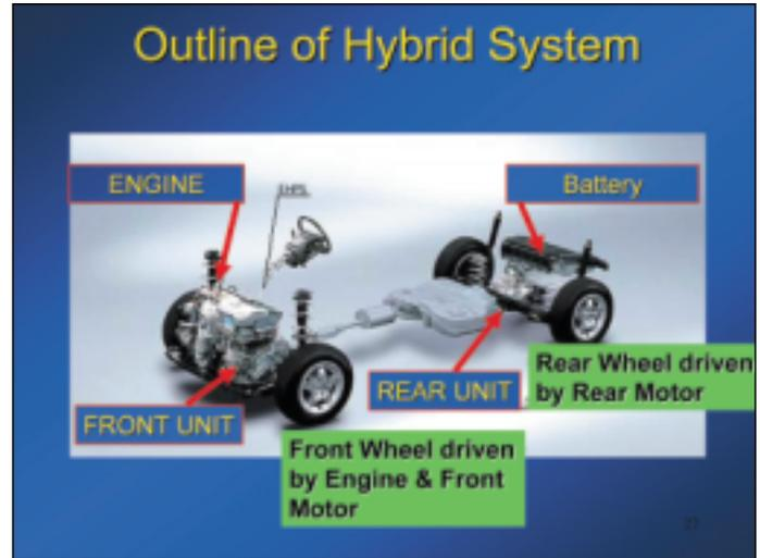
only by rear electric motor. There is no drive shaft between the front and rear units. Electronic unit controls the operation of the components in order to minimize gas consumption.
