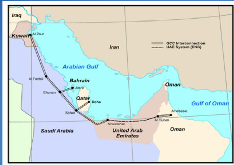
Here you can see the layout of the interconnection project. The route runs from Kuwait through Saudi Arabia to a place called Ghunan, from where we tap off to Bahrain, an island. So there is a submarine link. There is also a line branching off to Doha in Qatar. This is phase I. In this phase the 4 countries Kuwait, Bahrain, Qatar and Saudi Arabia will be connected.
