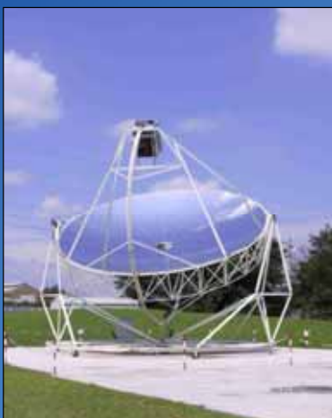
10 kW Dish Stirling solar generator system
