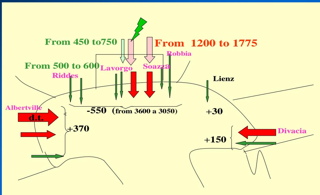
At 3.01.40h a flashover to a tree causes the opening of the Mettlen Lavorgo 380kV and consequently an overload (110%) of the Mettlen Soazza from 1200 to 1775 MW.
