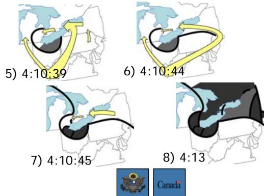
The cascade tripping lasts 10 minutes. Before the loss of Sammis-Star, the blackout was only a local problem in Ohio.
