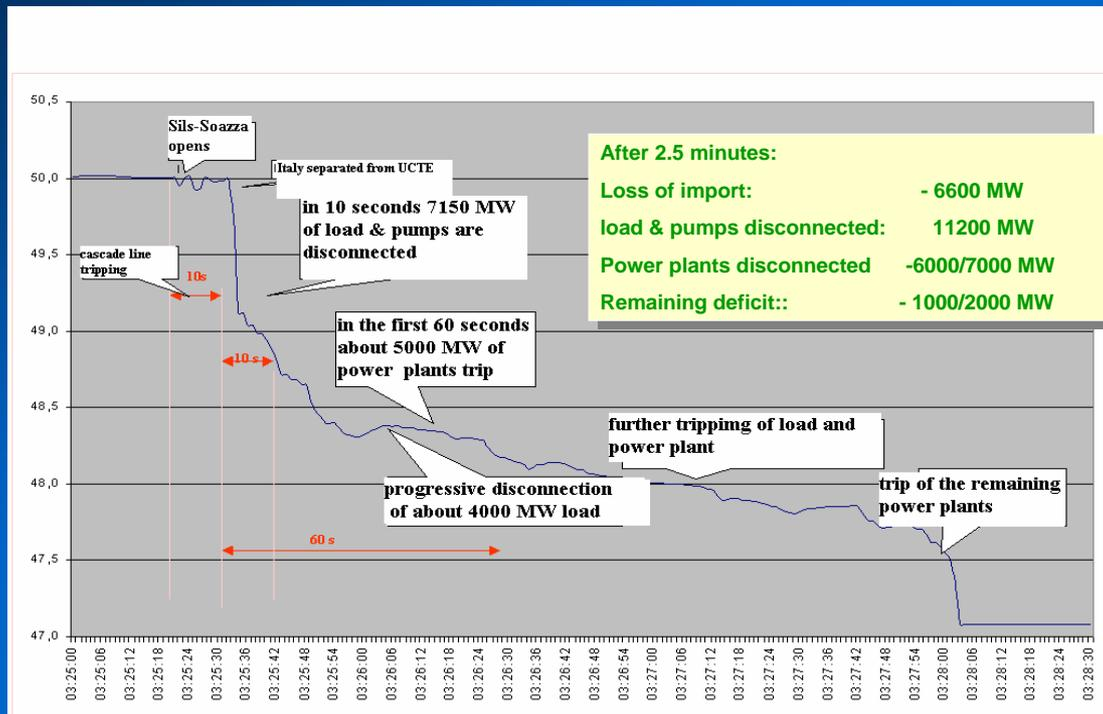
The transient of frequency lasts 2.5 minutes, during which there is a sudden decrease of the frequency in 10 seconds, accompanied by the disconnection of about 7.000 MW of pumps and loads, activated by frequency relays in accordance with the defence plans.
