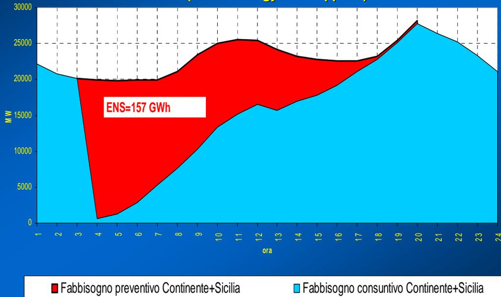
An example of a system that is not secure is given by the case of the Italian blackout of September 28, 2003. A cascade of lines tripping led to a disconnection of all the customers (Energy Not Supplied). All of Italy was out of power. The complete restoration took 18 hours.
