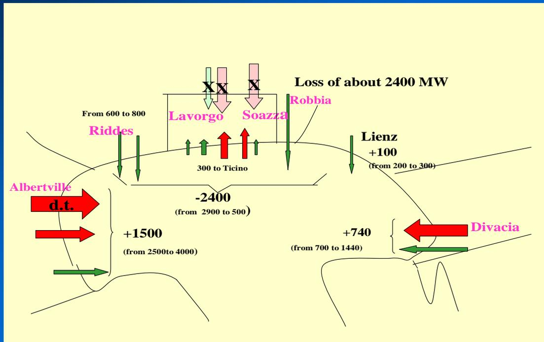
After the trip of the Sils Soazza line at 3.25.21h and of the Mettlen Lavorgo 220kV, 3 seconds later the Ticino area is isolated from the North and begins to import from Italy.
