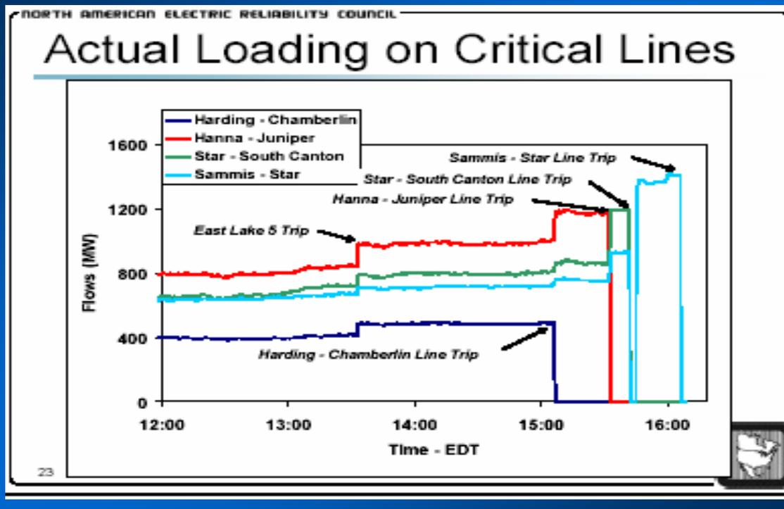
Similar to the Swiss line failure this figure shows that when a line trips, the power transits on the nearby lines increase. Consequently the high current heats the line conductors and causes an increase of the sag. The distance from conductors to nearby trees decreases and a flashover may occur that causes the opening of the line.
