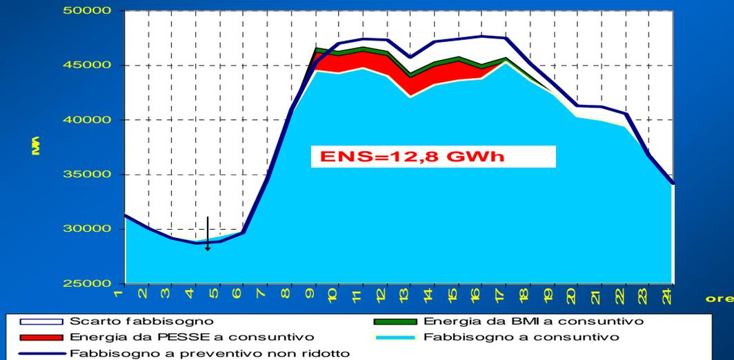
A typical example of a power system not adequate is shown in this slide that reports the energy not supplied (ENS, disconnection of customers) due to a lack of available generating capacity in front of a load demand higher than foreseen (long lasting period in Italy, July-August 2003, of high temperature and dryness). We had to cut off part of the load, indicated in red.
