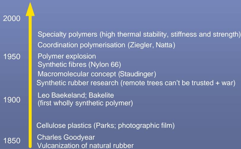
Before 1900, the polymers in use were from the nature (native polymers). These polymers were modified by some chemical reactions: vulcanisation (Goodyear); also the cellulose plastics.
