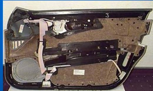
Another area of technology we see intruding into the conventional cable space somewhat is flexible circuit applications. I include in this flat cables and flexible printed circuits. The advantages of this technology are that it is lower weight, it can be easily packaged and it integrates well with either wiring or electronics or connectors.
